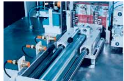
Typical application: Positioning sensing in automation technology; proximity sensors operate reliably and without wear.
