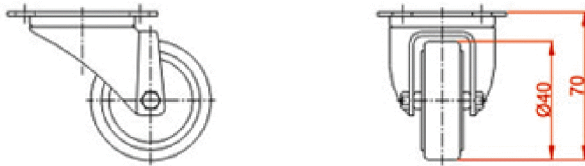
(Code:99) 45X45 Single Wheel With Brake Ø 50
