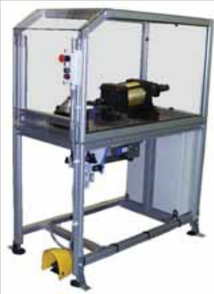
Automatic hot stamping of plastic seals by pigment transfer
