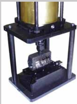
Steel boiler part marking with a customized numbering and integrated part support
