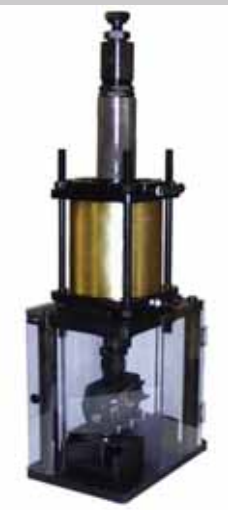
Steel boiler part marking with a customized numbering and integrated part support
